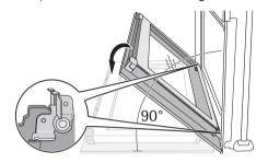
Loosen the clamp levers on both door hinges (A) completely.
